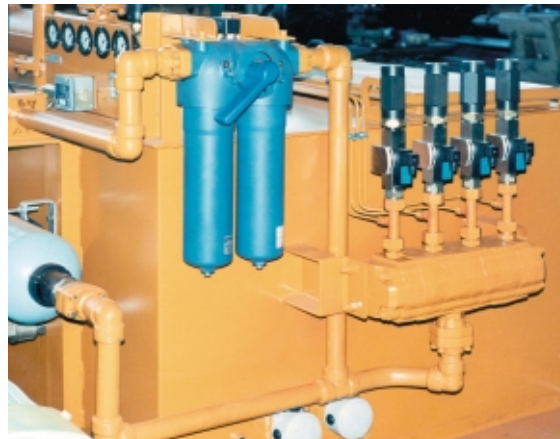
Fig. 10: Hydraulic power pack with duplex filter for the machine industry
