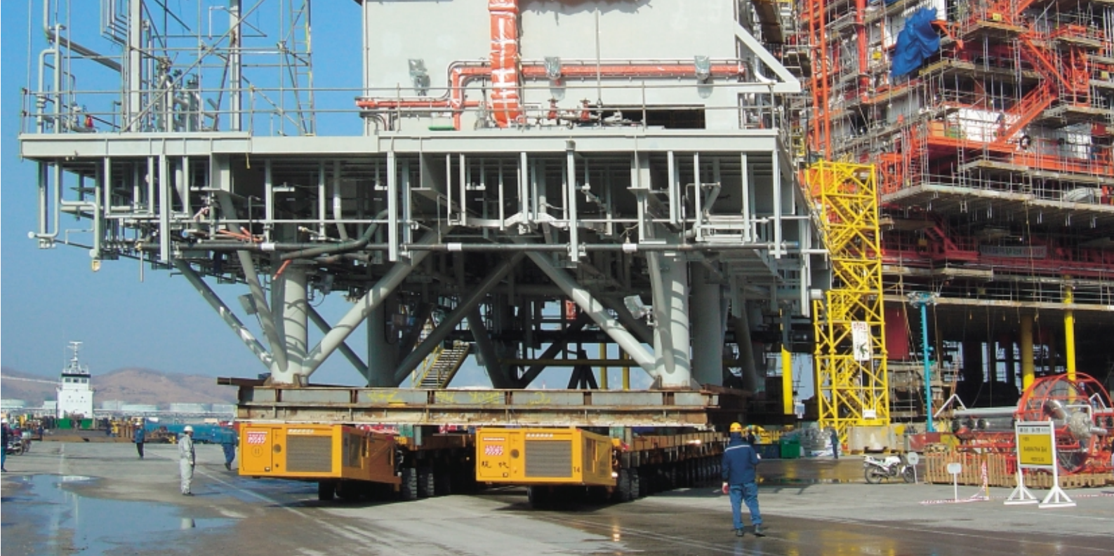
Fig. 8: Heavy load transport platform (Scheuerle) with MAHLE hydraulic filters
