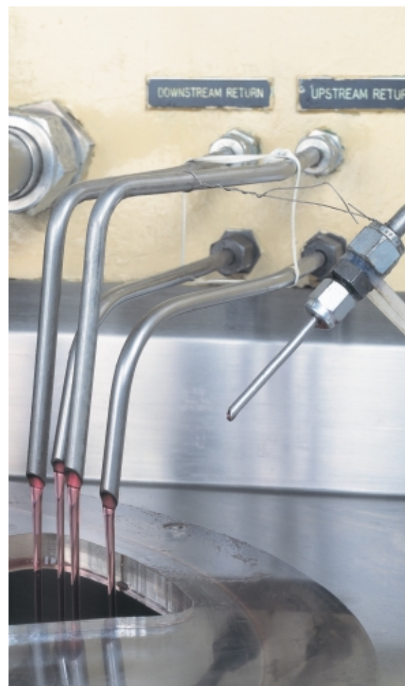
Fig. 48: Return lines on the multipass test rig
